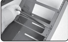
**STEP 2:** To fill gap, insert red portion of trim piece into gap starting on the right.
