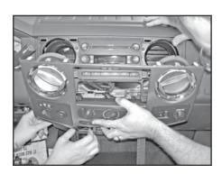
Replace upper panel making sure that the three connecters for the lower corner panels are threaded back through.
