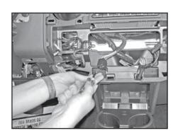
Remove the two center screws on the panel.
