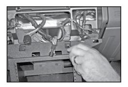
Replace 2 screws into upper center holes. (but do not tighten down)
