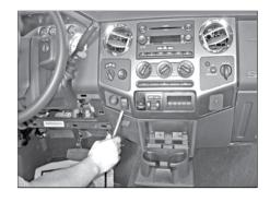
Use a flat head screwdriver to remove the left and right corners of the dash.
