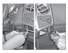
Remove the screws from the left and right side behind the corner panels.
