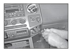
Replace the 2 screws located behind the 2 corner panels.
