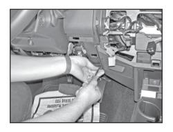
Remove the screw from the left side of the panel.
