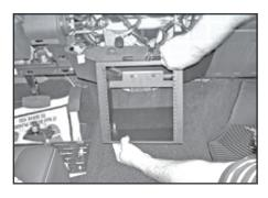
As levelers are adjusted shift console into place. Be sure outer holes line up (see pic. 18) Now tighten down all four screws from step 14 and 15.
