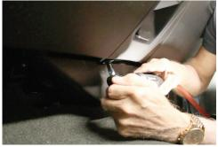
Remove (2) T15 scerws from under side of mini-compartment of OEM dash.
