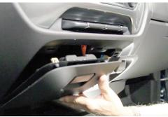
Pull mini-compartment away from OEM dash releasing clips.
