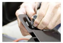
Remove OEM 12V outlet from minicompartment and relocate into Jotto Desk console.
