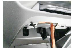
Insert bolt spacer/stud into slots into where clips on OEM mini-compartment.
