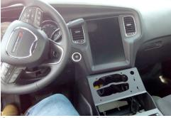
Secure console using OEM 8mm screws in the rear and OEM 10mm nuts in the front.
