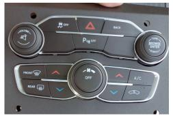
Slide module into provided cutout by aligning holes with studs on the backside of the console. Install provided nylock nuts to hold module into place.
