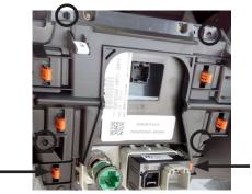
Remove Climate Control module by removing (4) screws from the back of the dash. Press out the (2) lower plastic spring clips (orange).
