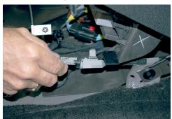
Disconnect wiring (4) harness for 12V and USB from OEM console.
