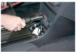
Remove forward OEM console plastic cover to expose OEM mounting points for aluminum floorplate. Remove (2) 10mm flange nuts. Nuts will be re-used.
