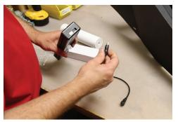
A 6 foot USB/Micro to USB cable is included. Secure one end into Brother printer and the other into the computer USB port.
