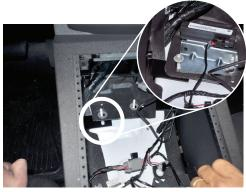
Remove 10mm OEM nuts from studs near proximity sensor. Pull up rubber pad placing front mounting bracket under pad. Replace rubber pad and proximity sensor and secure using OEM nuts.
