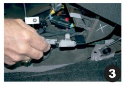
Disconnect USB connector from harness. Remove Ignition Proximity Sensor from plastic OEM console. Ignition Proximity Sensor will be remounted into Jotto Desk Contour Console.
