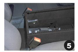
Relocate the Proximity Sensor to the mounting studs on the Jotto Desk Contour Console. Use the provided 8-32 nylon washers and place between console and sensor.
