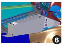
Console can now be adjusted forward and up to ensure a tight fit/finish with the OEM dash structure.
