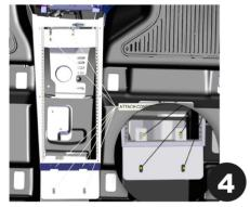
Secure top of console by using (2) M6-1.0 hex flange nuts.
