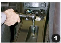
Remove forward OEM console plastic cover, then remove (1) 10 mm flange nut from center of plastic console. Nut will be re-used.
