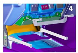
Attach the Upper Bracket to the dash with provided M4.2 x 1.41 x 2.0 screws. Tighten into place.
