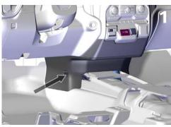
Remove 7 mm screw located on the driver side lower trim.
