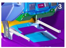
Attach the Lower Left and Lower Right Support Brackets to the OEM studs located by the main center dash supports. Loosely secure with provided flange nuts.
