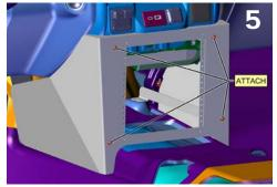
Place the Console into the vehicle. Secure in place by attaching the (4) provided screws through the front of the console and attaching to the previously installed Lower and Upper Brackets. Tighten flange nuts on Lower Support Brackets to complete installation.
